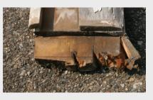
TRADITIONAL WOOD FRAME Susceptible to rotting, warping, and decay
